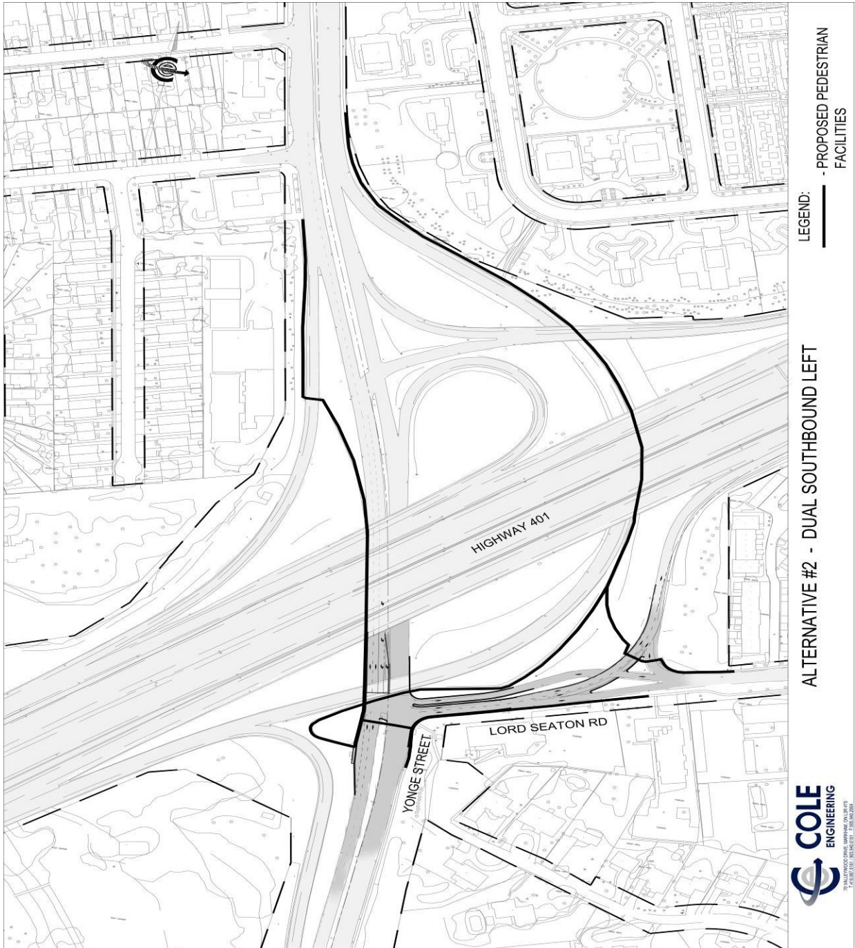
Figure 2.1 - Alternative #2: Dual Southbound Left
