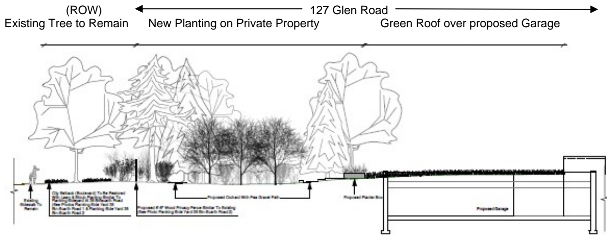
Elevation B1-B1 (reference Landscape Plan) West-East view through mid-point of property including proposed orchard and green roof over parking structure
