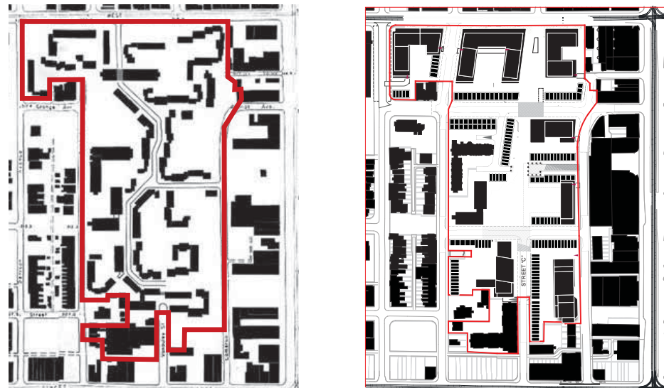
Figure 5: Figure ground of the Site pre-1986 (left) and the Site Proposed (right)
