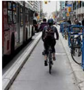
Cycle Track separated by curb stones.
