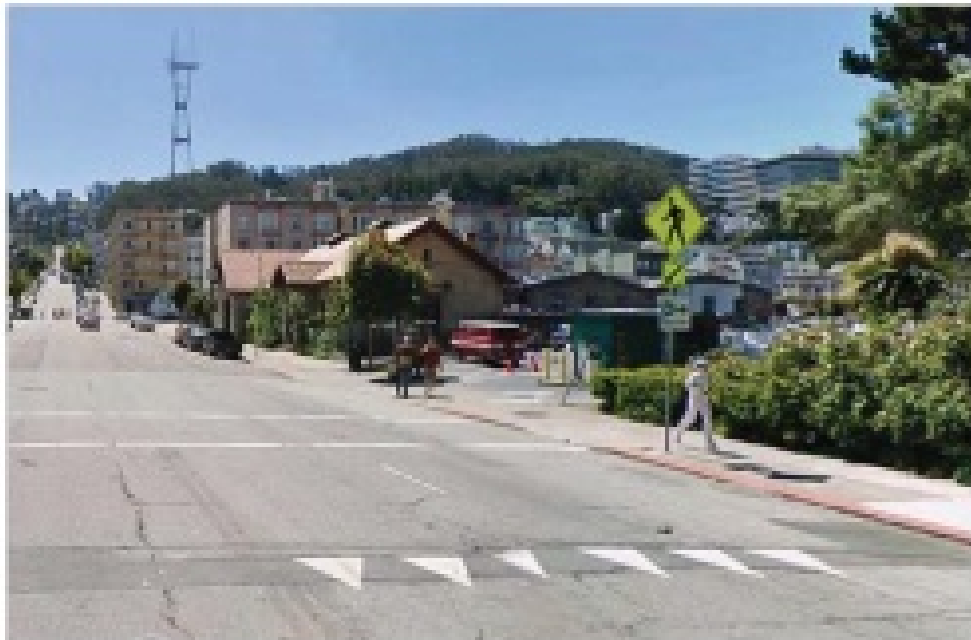
Figure 7: San Francisco yield lines in crosswalk (Photo Credit: Timothy Papandreou, San Francisco Municipal Transportation Agency)
