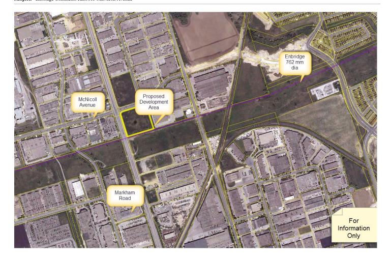
Enbridge Pipelines Inc. (Enbridge) does not have facilities within the scope of the proposed project. As per the attached aerial photo, Enbridge owns and operates a "762 mm dia." pipeline near the subject lands approximately 20 m from the subject lands.
