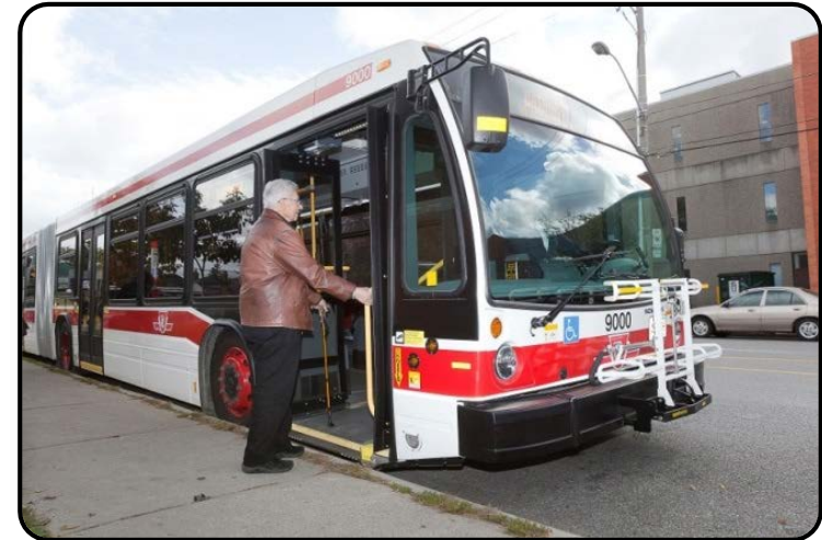
High-Floor Buses with Steps and Lifts Replaced with Low-Floor Ramp Buses
