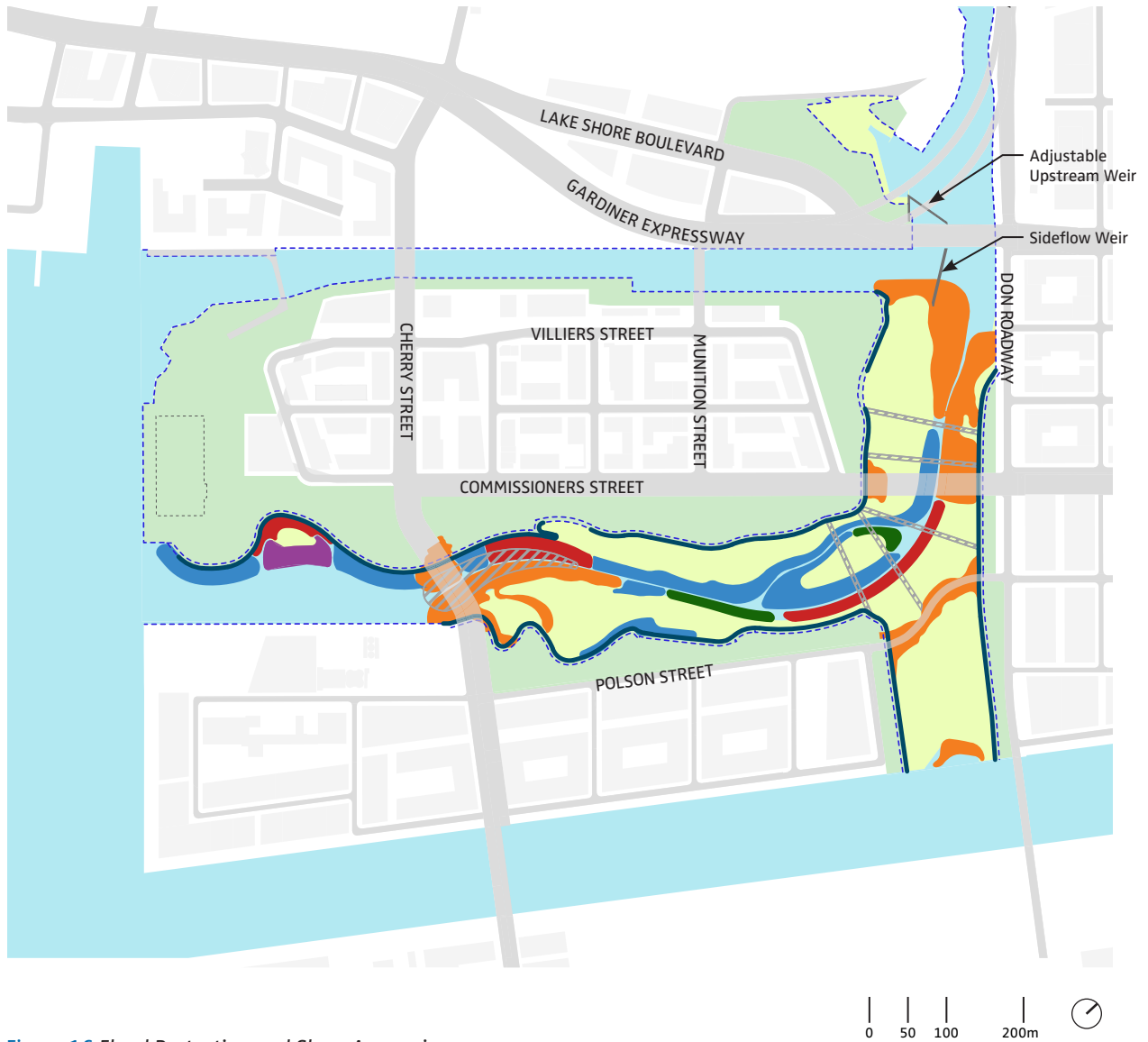
Figure 16 Flood Protection and Slope Armoring
