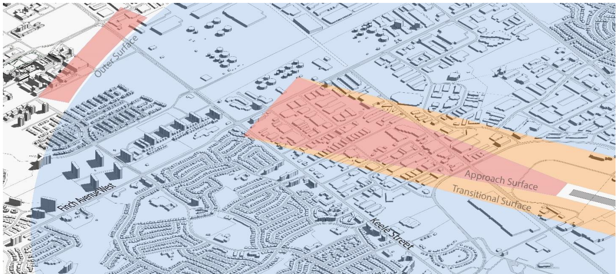
Figure 2 TP312 4 th Edition – Elevated Perspective of composite OLS surfaces.
