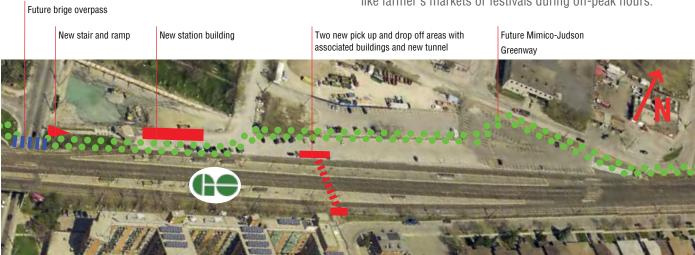
Figure 3: Diagram of future station improvements shown in red. The Mimico-Judson Greenway and bridge overpass should be provided and are shown here for illustrative purposes.
