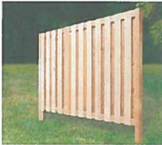
Treated wood 6 x 8 ft privacy fence panel with 2 x 3 in crossers. 1 in x 6 in x 6 ft boards Panel finished both sides.
