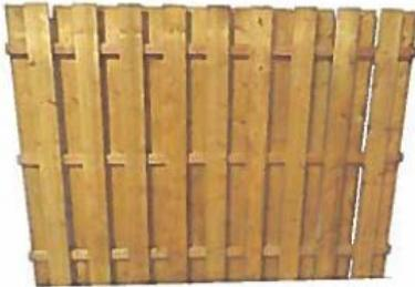
Treated wood privacy panel with alternating shadow box style and flat top, total length 96", 3- 2x3 crossers for added support, 1x6x6 fence boards, finished on both sides, double nail construction.
