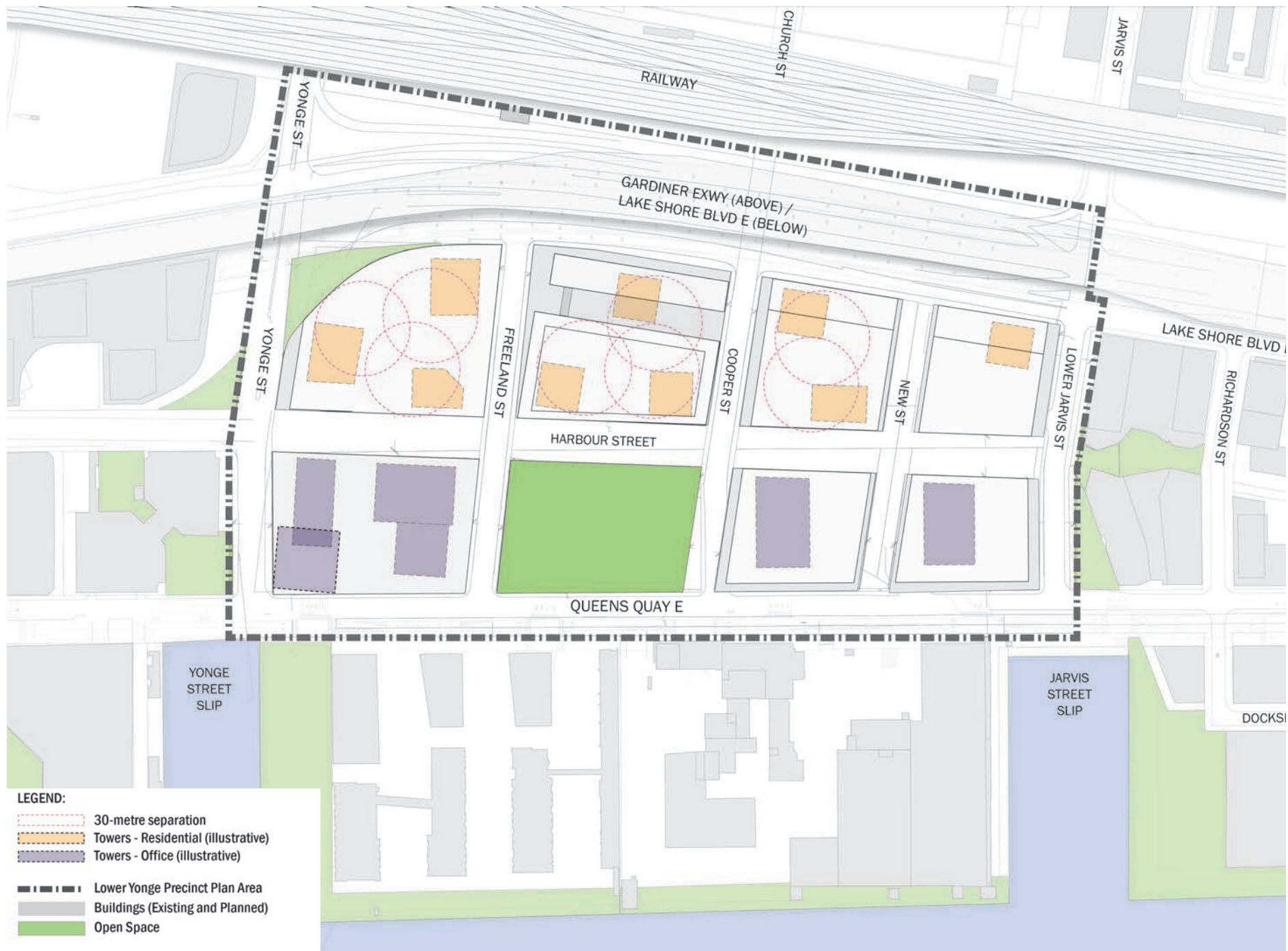
Figure 5.31 Tower Location (illustrative) and Tower Separation
