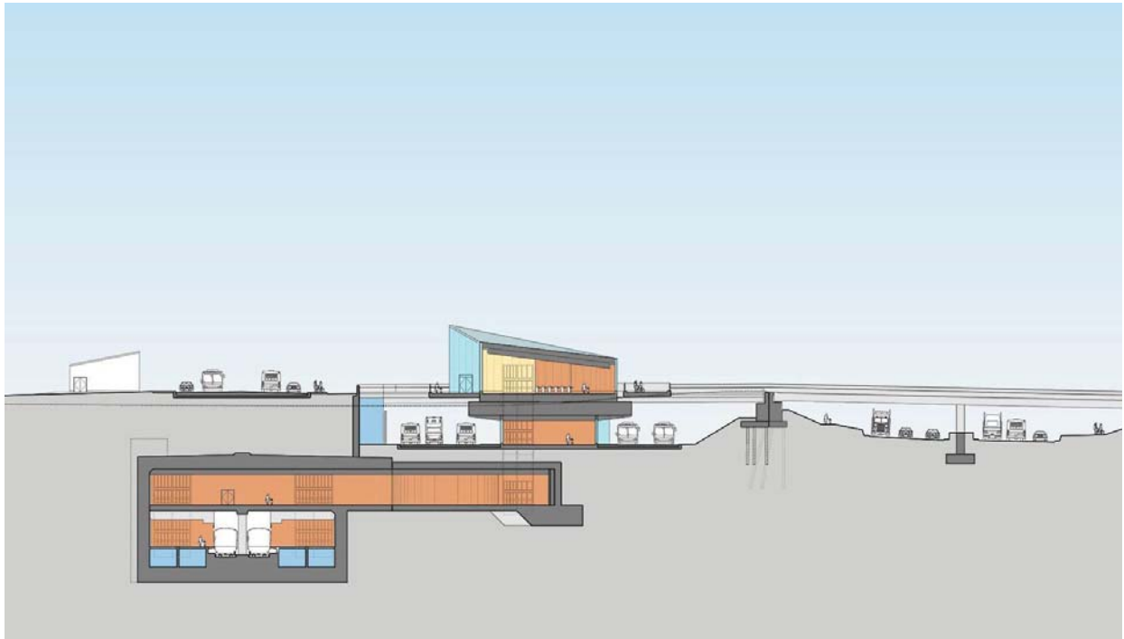
Figure 4: Scarborough Town Centre Station Cross Section of Subway and At-grade Bus Station
