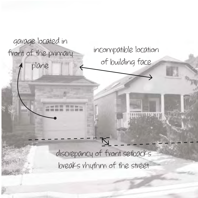
Figure 50 Incompatible building face
