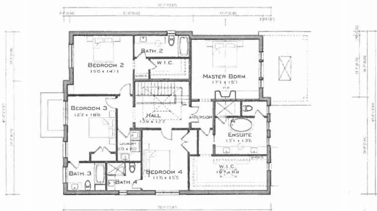
SECOND FLOOR PLAN SCALE: 1/8" = 1'-0" AREA = 2,503.27
