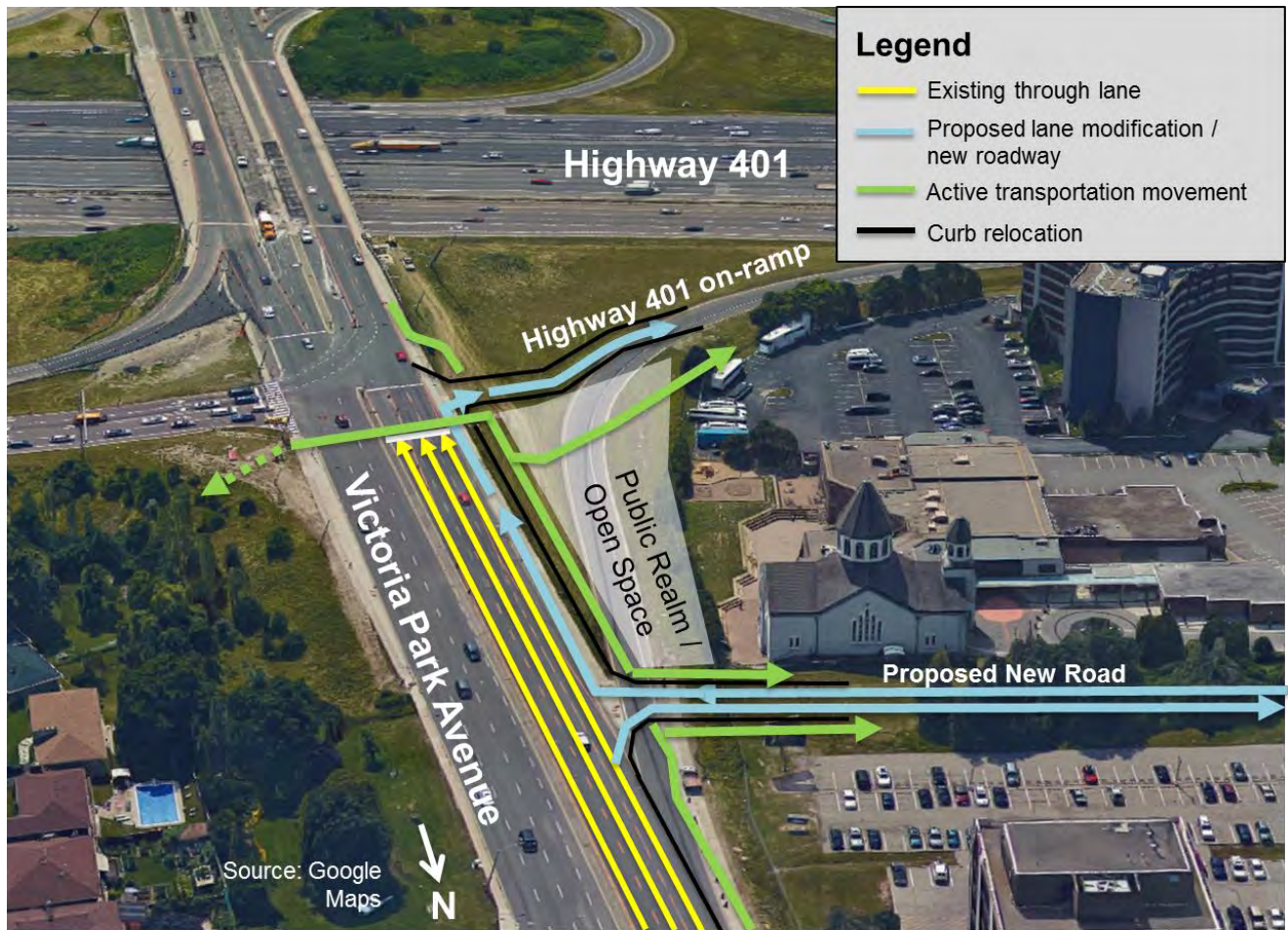
Exhibit 10-12: Conceptual proposed improvement at Victoria Park Ave at Highway 401 WB Ramp – Plan View
