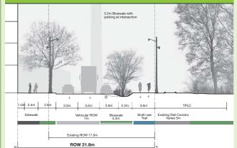
Realign Unwin Avenue and provide one-lane of traffic in each direction (two-lanes total) while optimizing carrying capacity and providing enhanced pedestrian and cyclist amenity and integrated stormwater management. Alignment in the vicinity of the Hearn/PEC to be confirmed in Phase 3 of the Municipal Class EA process.
