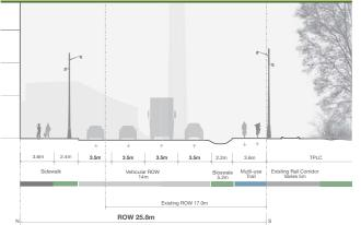
Maintain the existing alignment and capacity and improve the existing onelane Bailey Bridge by providing a two-lane bridge across the circulating channel. Realign Unwin Avenue and provide two-lanes of traffic in each direction (four lanes total) with improved pedestrian and cycling amenity and some integrated stormwater management. Alignment in the vicinity of the Hearn/ PEC to be confirmed in Phase 3 of the Municipal Class EA process.
