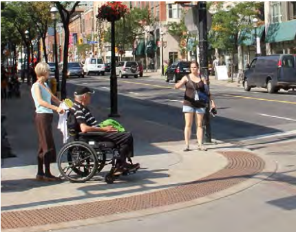
Reduced corner radii help to slow turning traffic.
