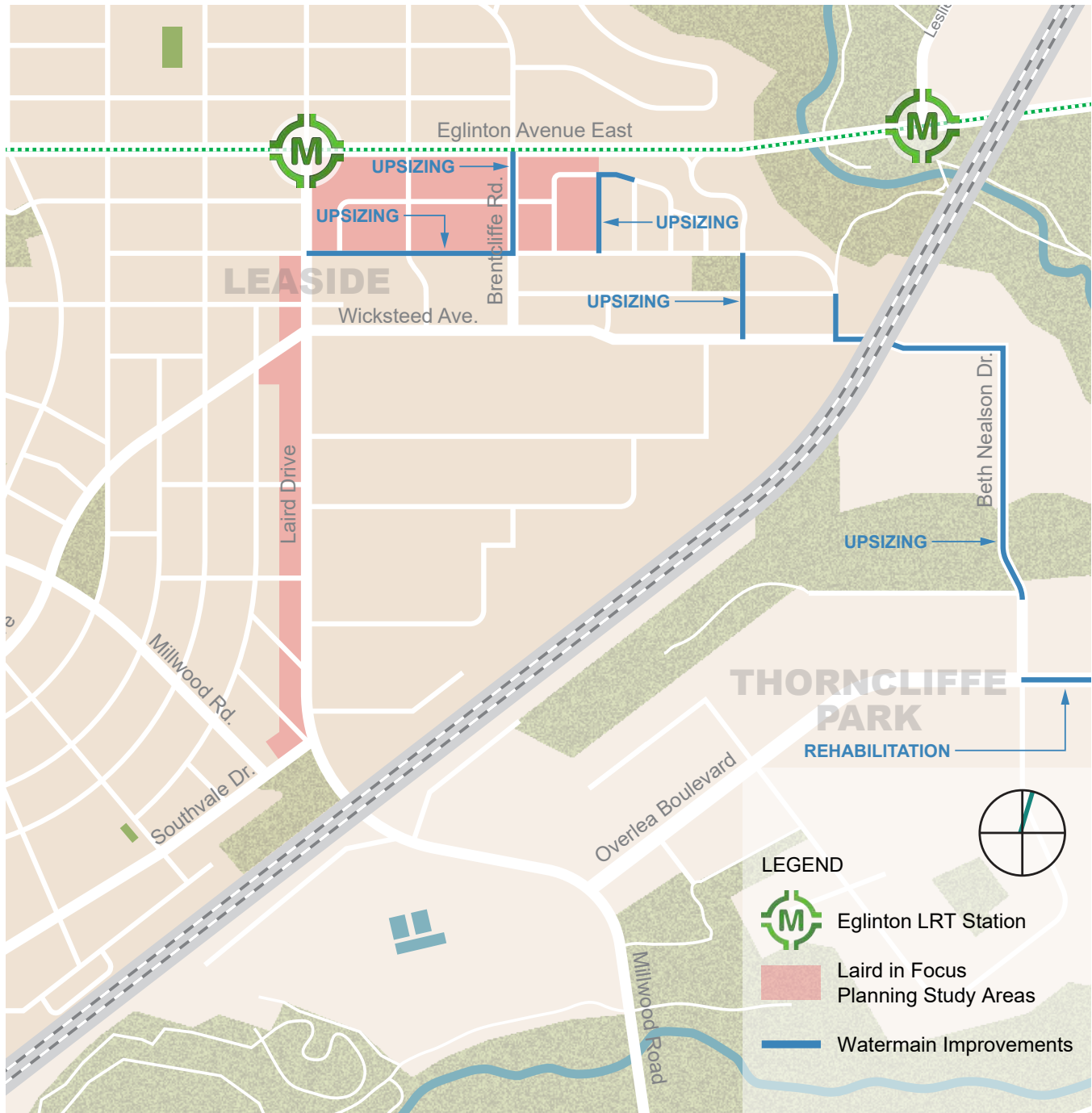
Location of identified watermain improvements necessary to support development intensification
