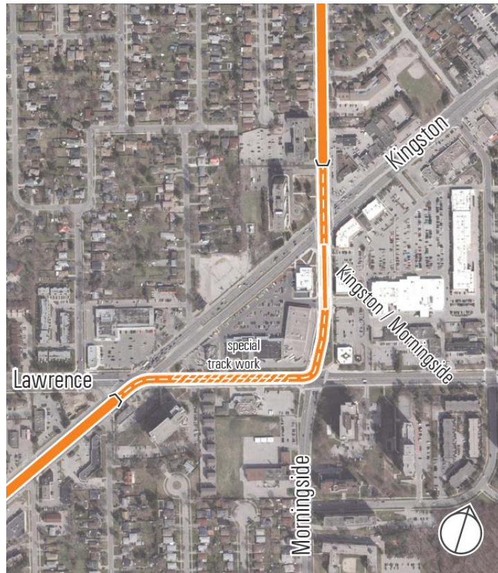
Figure A3-5: Lawrence/Morningside Single Stop below-grade (tunnel)
