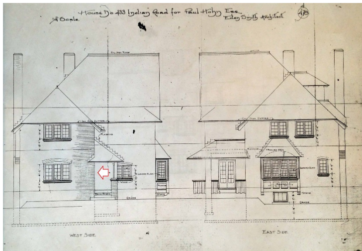
4a. Architectural Drawing, West (left) and East (right) Elevations: showing the location of the main entrance on the side of the L-wing (arrow) and the open verandah on the rear
