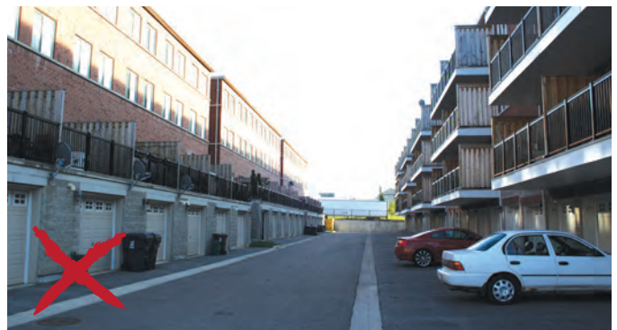
Avoid lanes like the above without accommodation for utilities, landscaping and quality design, especially when amenity spaces overlook the area.
