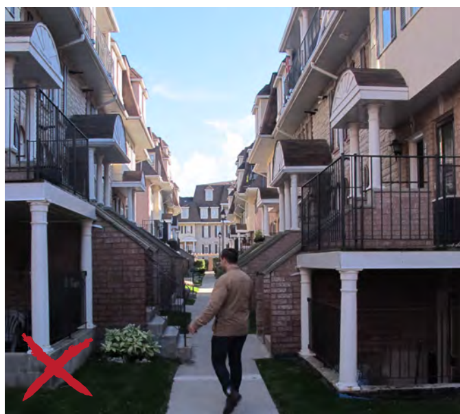
Avoid excessive projections such as stairs, porches, stoops, canopies, and private amenity spaces into pedestrian mews and front yard setbacks.
