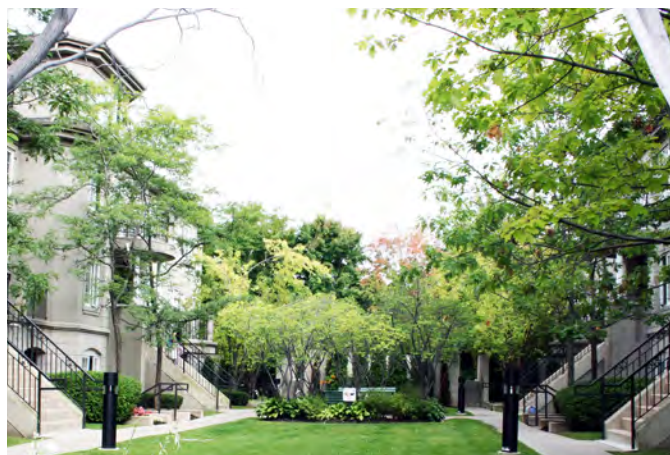
Sufficient facing distance allows for attractive landscaping between buildings, good access to sunlight and sky views. Avoid more than 3-5 steps up or 8-9 steps down to the units to further improve the shared spaces between buildings.
