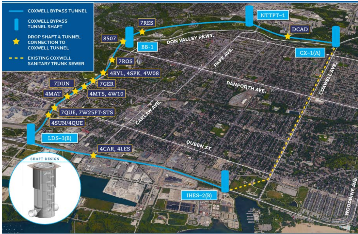
Figure 2. Photograph showing the alignment of the Coxwell Bypass Tunnel and Location of the Associated Wet Weather Flow Connections.
