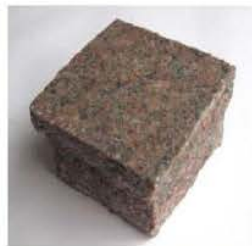
Royal Canadian Red Size: 90 x 90x80mm Top finish: Light waterjet Side finish: Split Joints: 5-8mm joints
