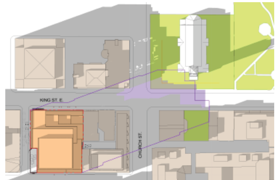
Shadow study (IBI Group Architects). The purple line indicates the extent of shadows from a previous submission. The purple hatch shows the extent for the current submission.
