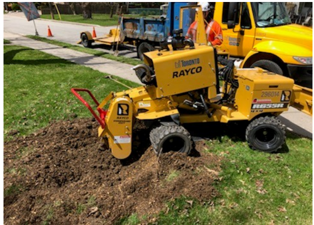
A Crew Member Using a Stump Grinder to Take Out a Tree Stump
