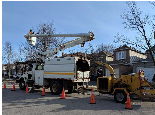
A Two-Person Crew with an Aerial Lift Bucket and a Brush Chipper for Tree Pruning Service
