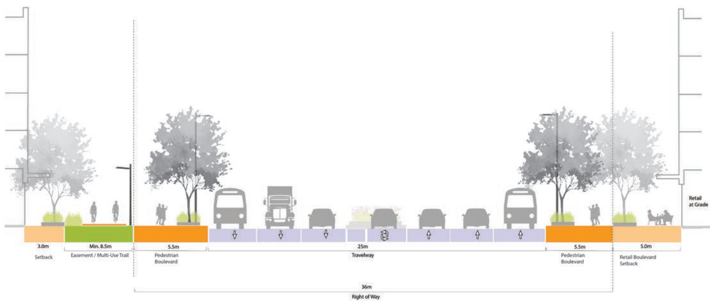
The Queensway Section Option 2: Multi-use Trail in Enbridge Easement
