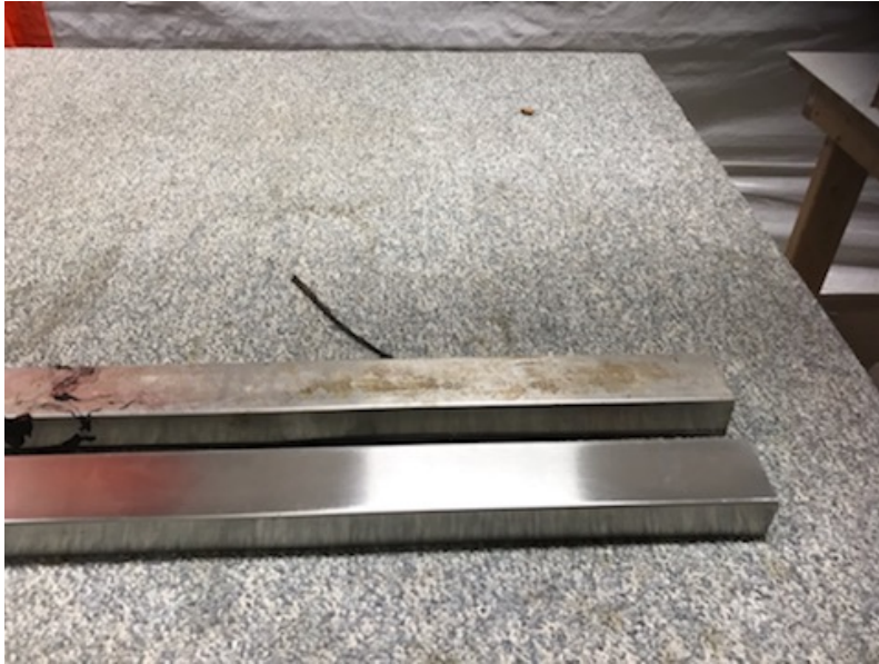
Figure 7: Uncleaned (top) and manually-cleaned (bottom) aluminum snap caps
