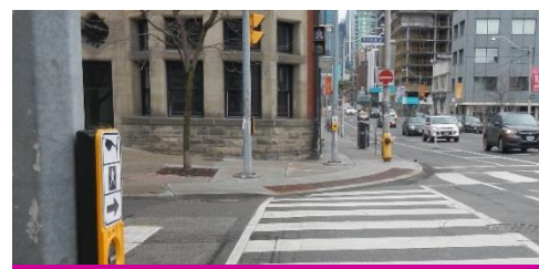
Accessible Pedestrian Signals
