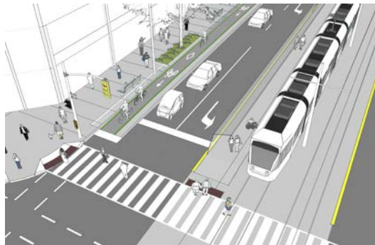
Centre-Running Transit Option E: Centre median stop
