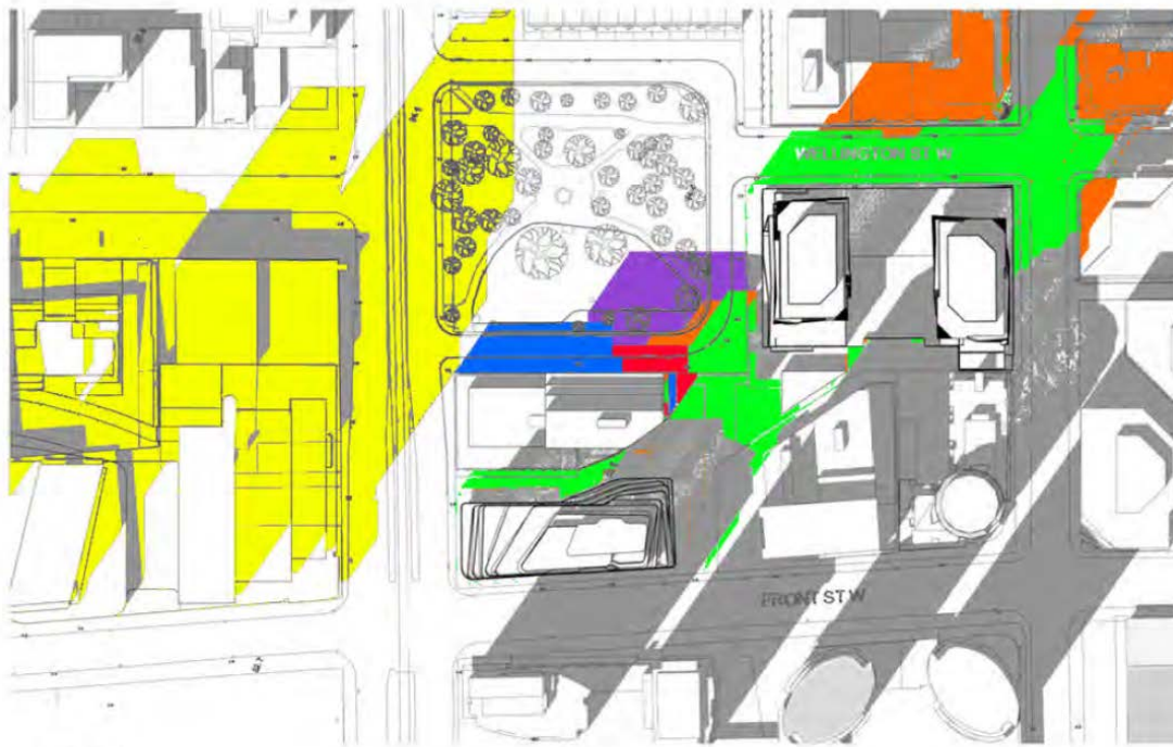
Shadow study of the current proposal (the net new shadow cast by 14-storey office building on March 21 is shown in purple)
