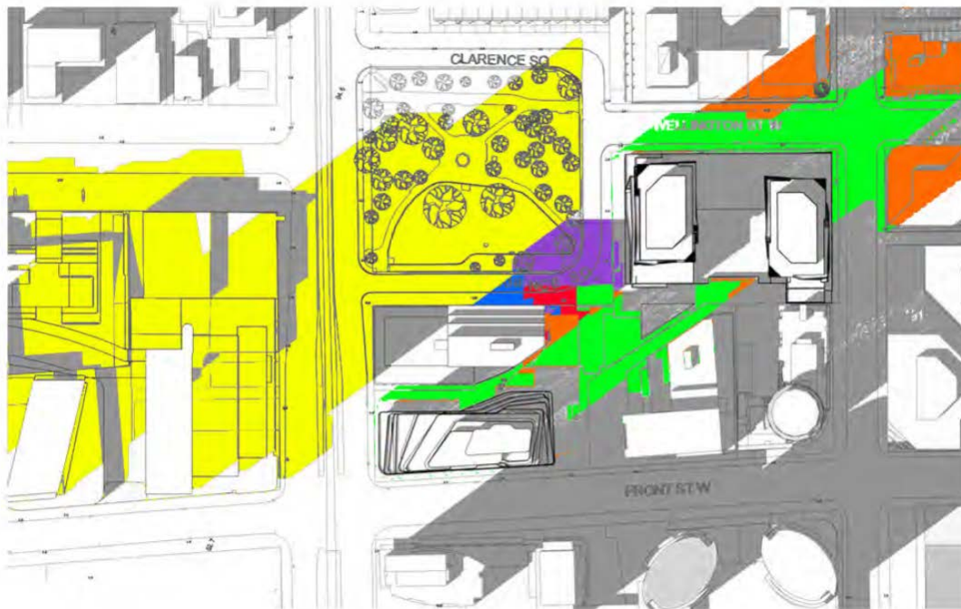
Shadow study of the current proposal (the net new shadow cast by 14-storey office building on March 21 is shown in purple)
