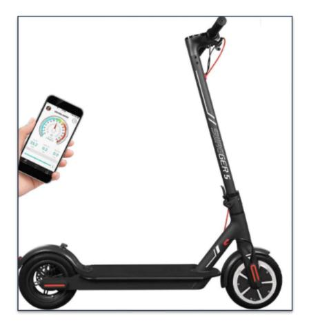
An e-scooter is a two-wheeled device the rider stands on, holding a handlebar, see picture. It has a battery and can travel at a speed of 24 km/hour using a throttle.
