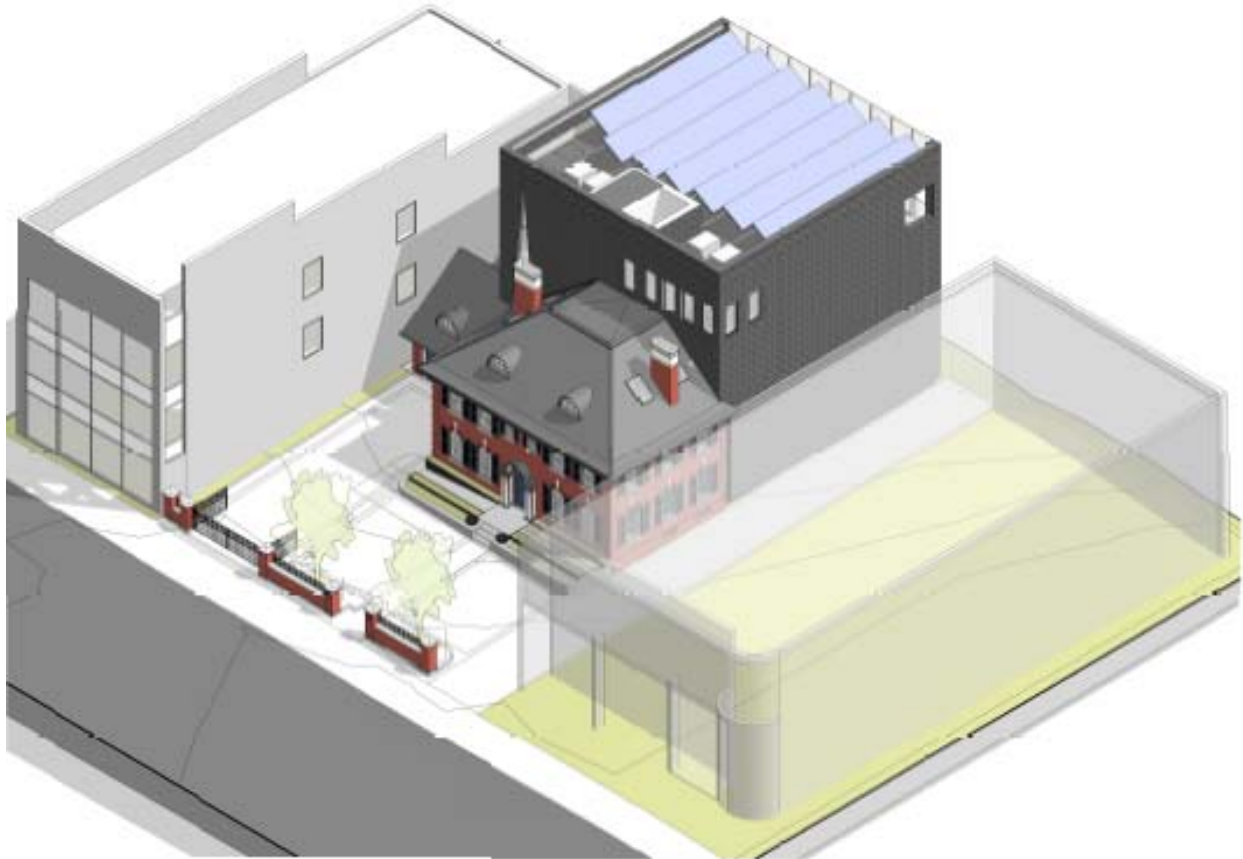
Axonometric view of the existing house-form heritage building and proposed rear addition as seen from above to the southwest in relation to adjacent buildings (Dewson Architects)
