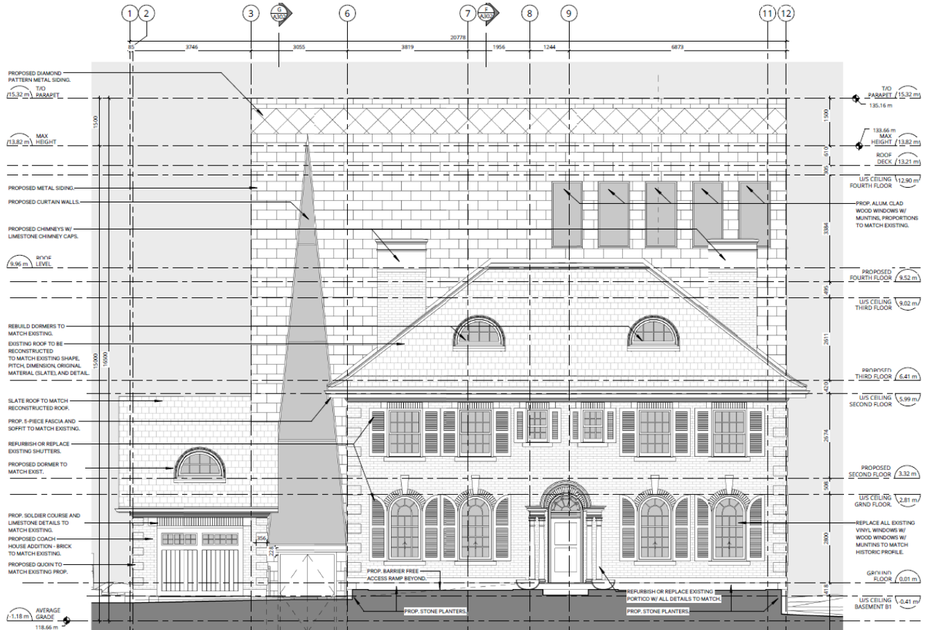
Proposed west (front) elevation of the building at 1067 Yonge Street, showing the heritage house-form building set in front of the proposed rear and side addition (Dewson Architects)
