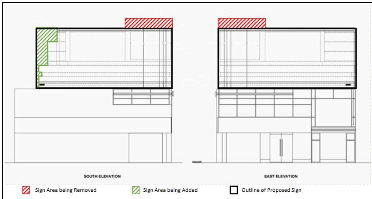
Figure 3 - Comparison of existing sign and proposed sign (staff rendering made in consultation with applicant)
