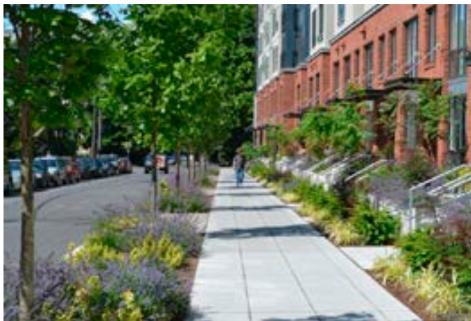
Boulevard treatment for a narrower and quieter residential street with street trees in soft landscaping (Seattle, Washington, USA)
