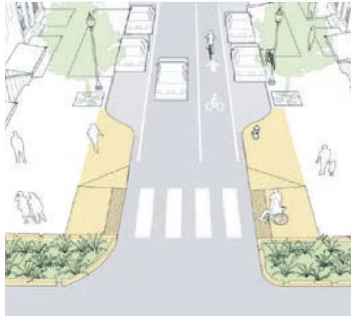
Corner extensions at intersections shorten pedestrian crossings and promote pedestrian safety (Source: Urban Street Design Guide; NACTO.org)
