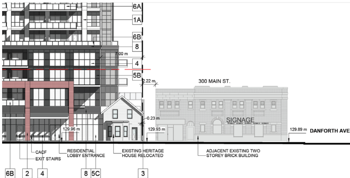
Detail of East Elevation (North-east corner of site adjacent to relocated heritage property - gable missing from south elevation of relocated house)
