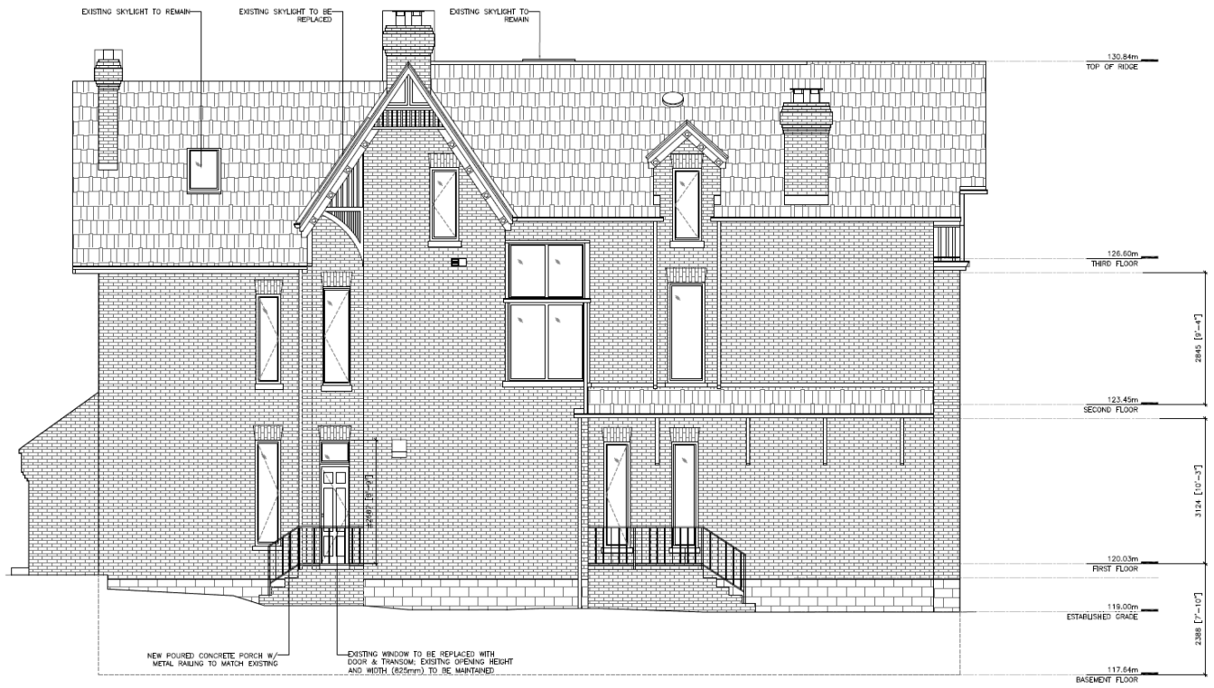
North elevation drawing showing the location of the proposed secondary north entrance and new porch.
