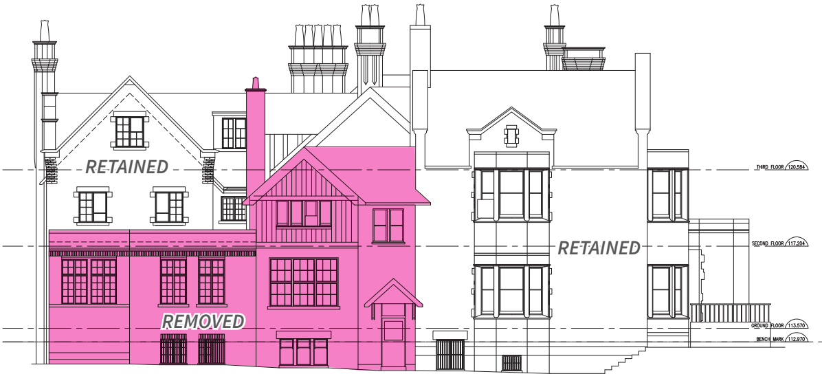
Retention and removal areas on the west elevation (ERA, 2018).
