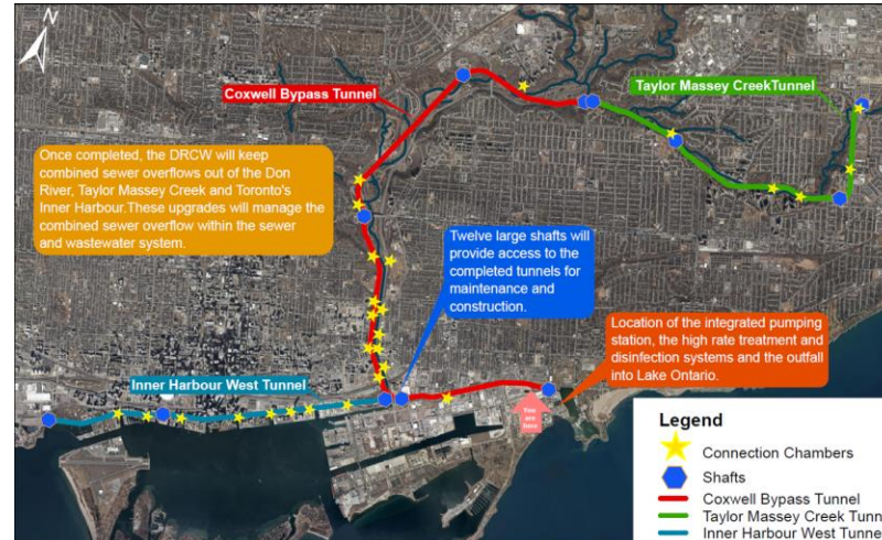
Don River and Central Waterfront & Connected Projects Wet Weather Flow System to improve river and Harbour water quality: 22 km tunnel system consisting of three integrated tunnels Coxwell Bypass (stage one), Taylor Massey-Creek and Inner Harbour Tunnels
