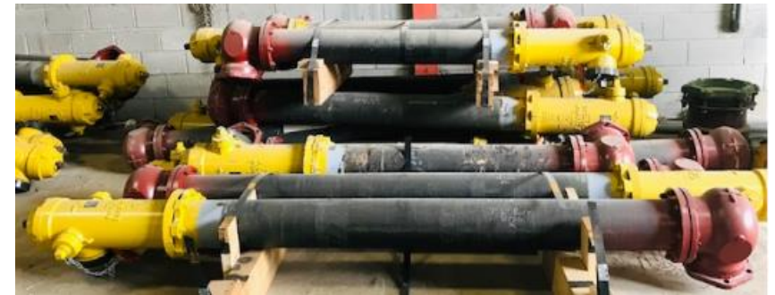
Fire hydrants, Disco Yard
