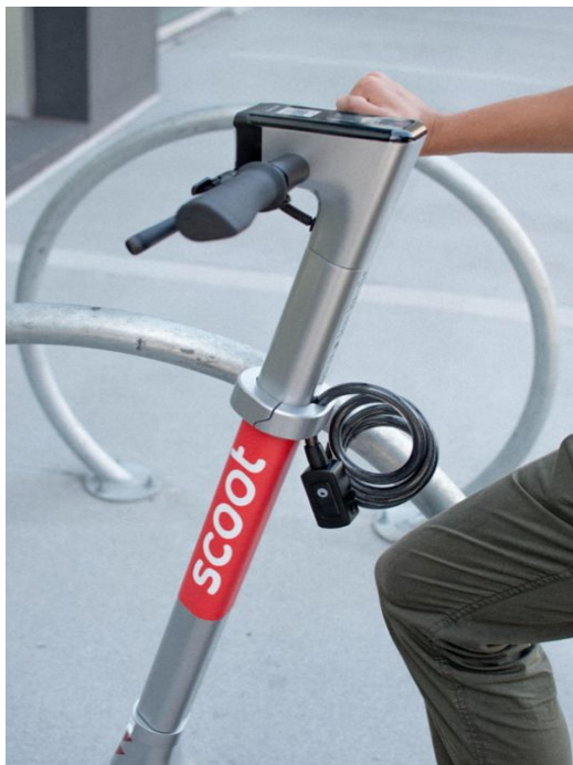
(Image of a e-scooter locked to a bike rack via an integrated electronic lock attached to the e-scooter)
