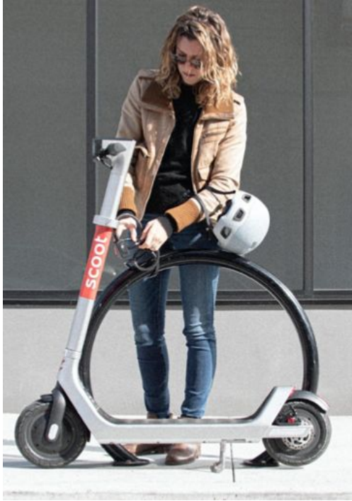
(Image of a woman locking an e-scooter to a bike rack via an integrated electronic lock attached to the e-scooter)
