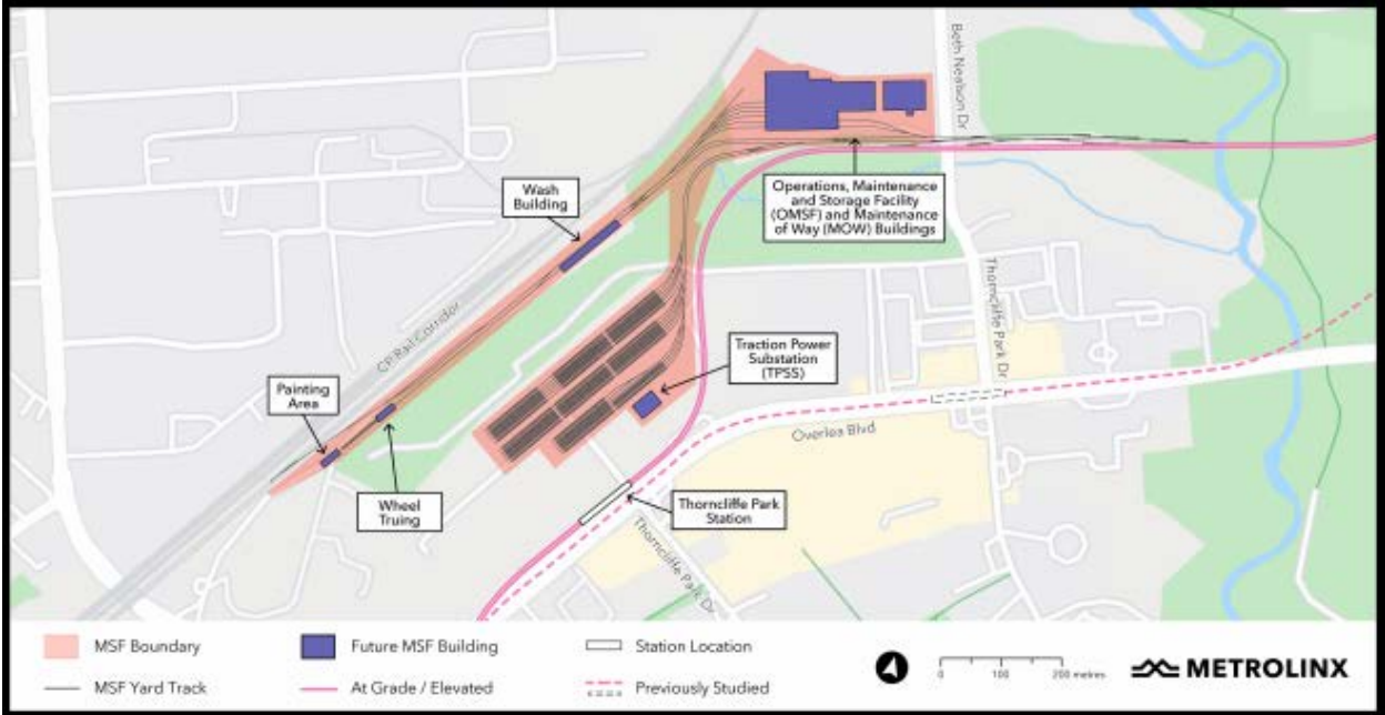
Figure 6. Metrolinx Proposed MSF Site Location (Source: Metrolinx).
