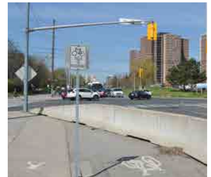
Figure 30. Varying materials and signage to indicate split between cycling and pedestrian pathways
