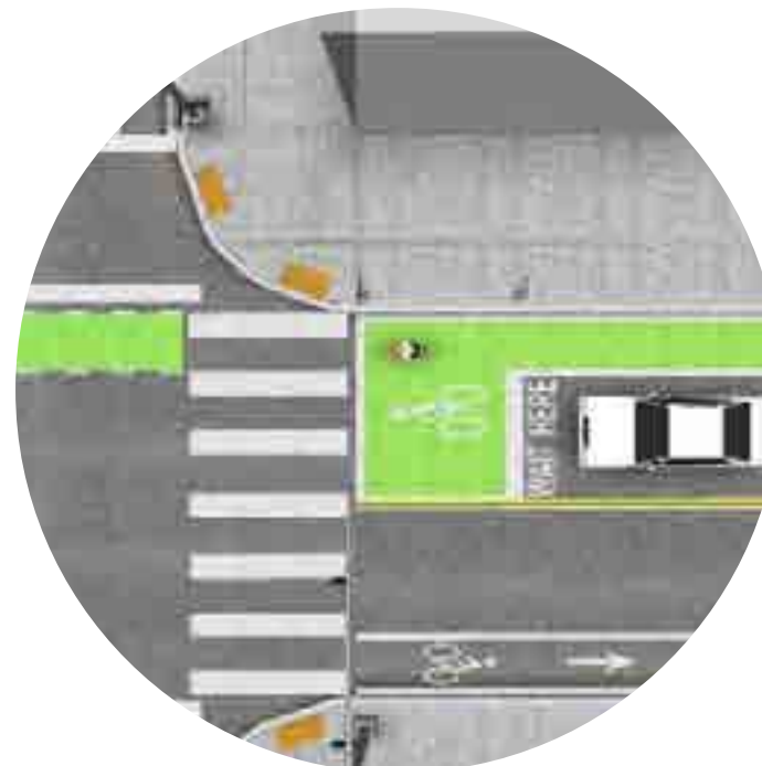
Figure 196. Bike box at a signalized intersection with a bike lane approach (NACTO Urban Bikeway Design Guide)
