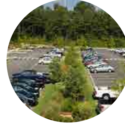
Figure 225. Surface parking lot retrofitted to reduce paved hardscaped area
