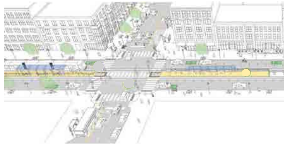
Figure 249. Example of streetwall for a ‘Downtown Median Transit Street’ (diagram from NACTO Transit Guide)
