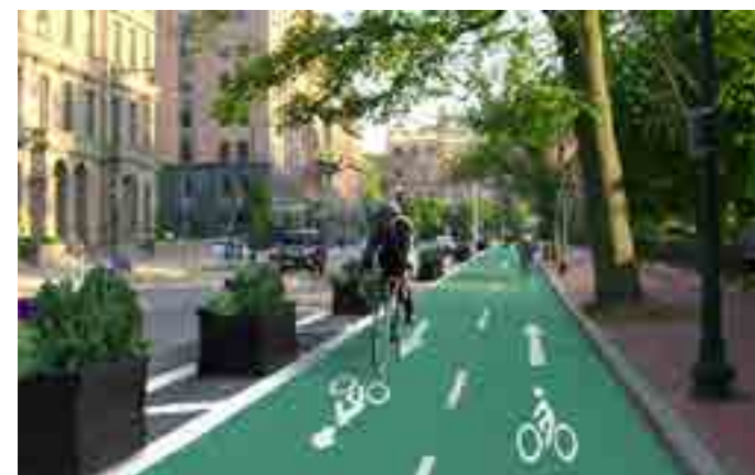
Figure 179. A distinct, two-way dedicated cycling trail, buffered from motorized vehicles and sufficiently separated from pedestrians (Charlotte, US)
