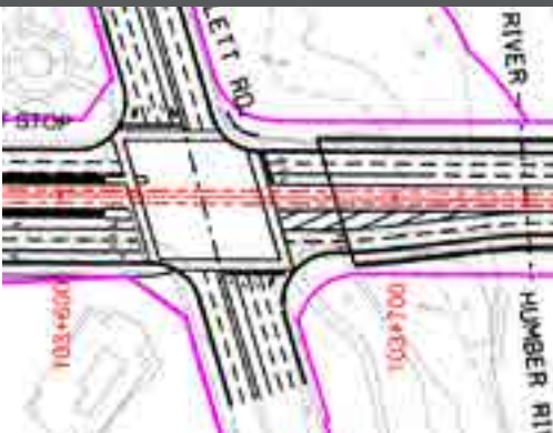
Figure 328. Revisions to the alignment along Humber Bridge resulting in the need for bridge widening
