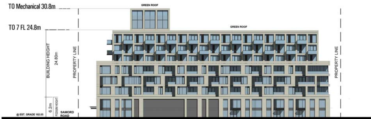
West Elevation - 7 Storey Residential Building
