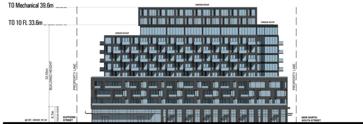
North Elevation - 9-10 Storey Mixed Use Building
