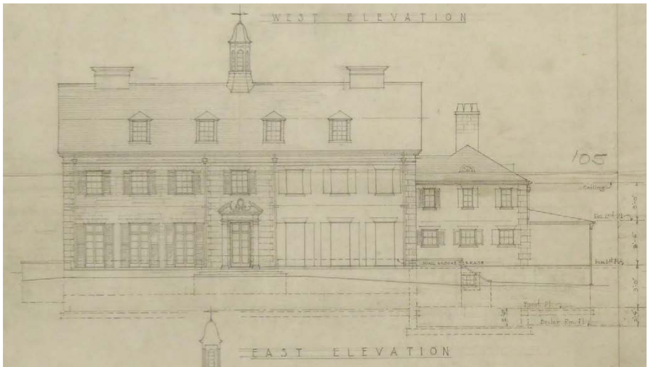
10. East Elevation drawing showing the garden side with its French doors opening to the terrace, and, to the right the end wall of the service-garage building
