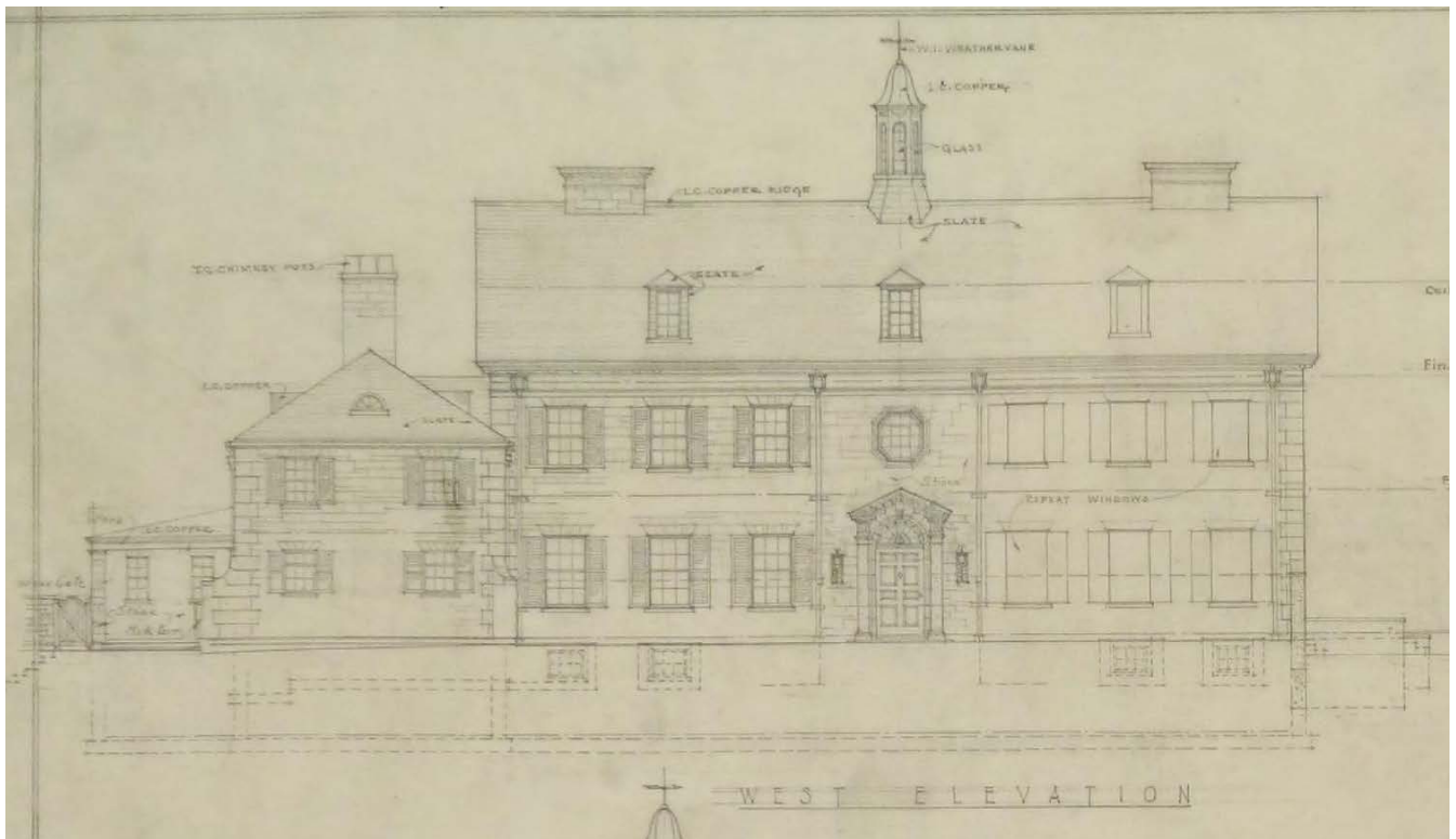
9. West Elevation drawing showing the principal entry elevation of the main house (right) and the service-garage building (left) with its single-storey extension and gate (far left)
