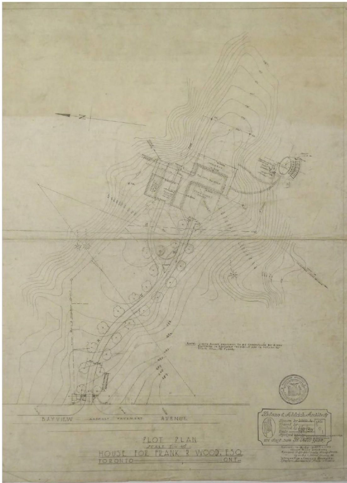
6. 1930 Site Plan of 2365 Bayview Avenue, by Delano & Aldrich, showing the contours of the land and the alignment of the site plan in relation to the ridge in the design of the driveway from Bayview Avenue in the west and the arrangement of the house and outbuildings to the landscape
