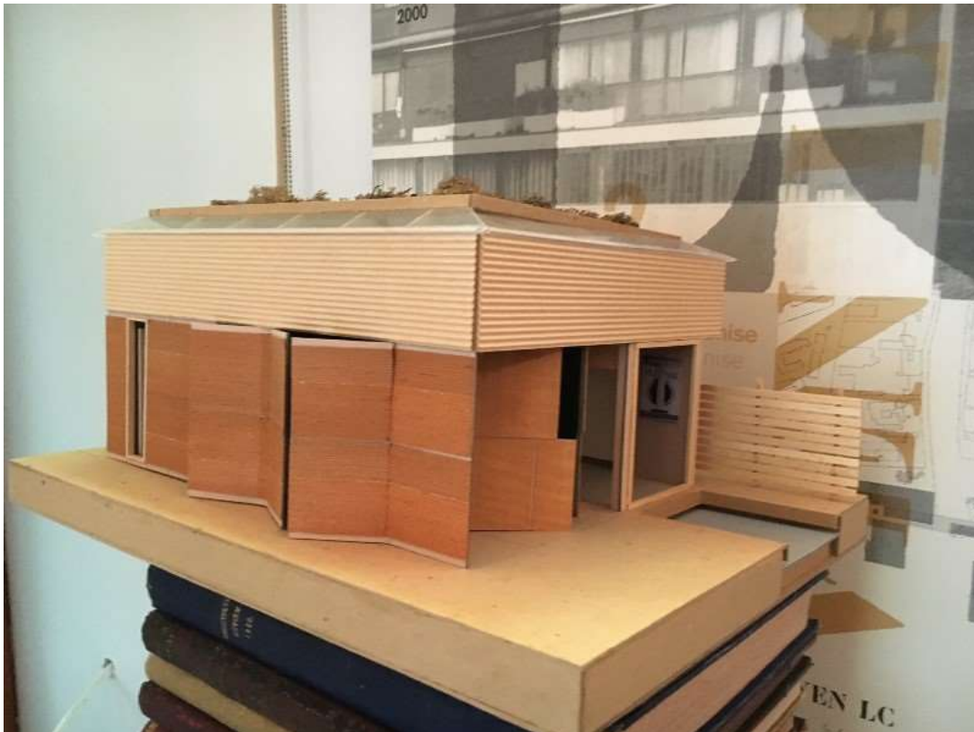
Figure 54. Model of the studio, constructed by Robert G. Hill, showing the scheme as constructed and showing the opening doors for the garden storage on the north elevation, with the cladding materials, skylights, green roof and design of the west elevation. (Photo credit: Heritage Planning, 2021)
