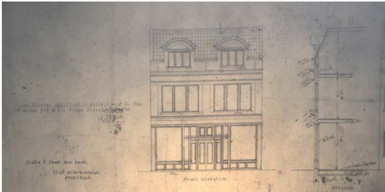
8. 1924 architectural drawing of 516 Yonge Street's east elevation, by architect Oluf Albrechtsen. This drawing shows the alterations made to the building in 1924, including changes to the storefronts, second storey window openings, dormers, and roof profile. (City of Toronto Building Records)
