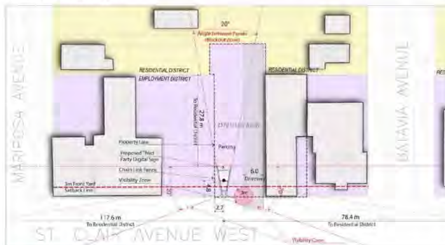
Figure 6: Visibility Zone shown on Subject Site
